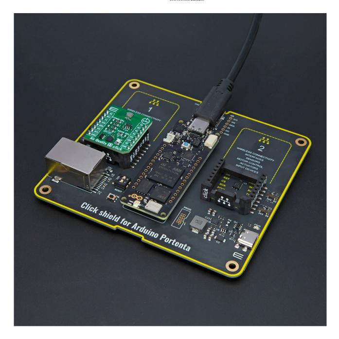
When the USB is connected to the Portenta board, the PWR diode will glow Green, and at this setup, the Portenta H7 baseboard itself will be supplied, and it will provide power to the Click Shield, including all mikroBUS™ sockets.
