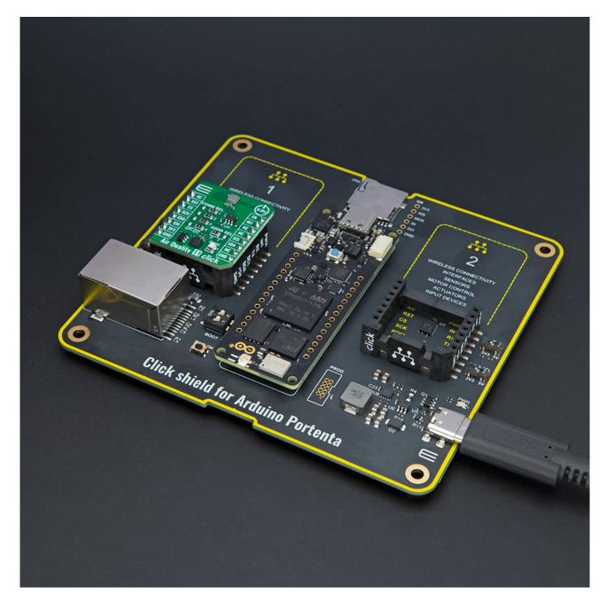
When the USB is connected to the Click Shield, the PWR diode will glow Blue, and at this setup, the connected Portenta baseboard and all mikroBUS $^{\text{m}}$  sockets will be powered from it.
