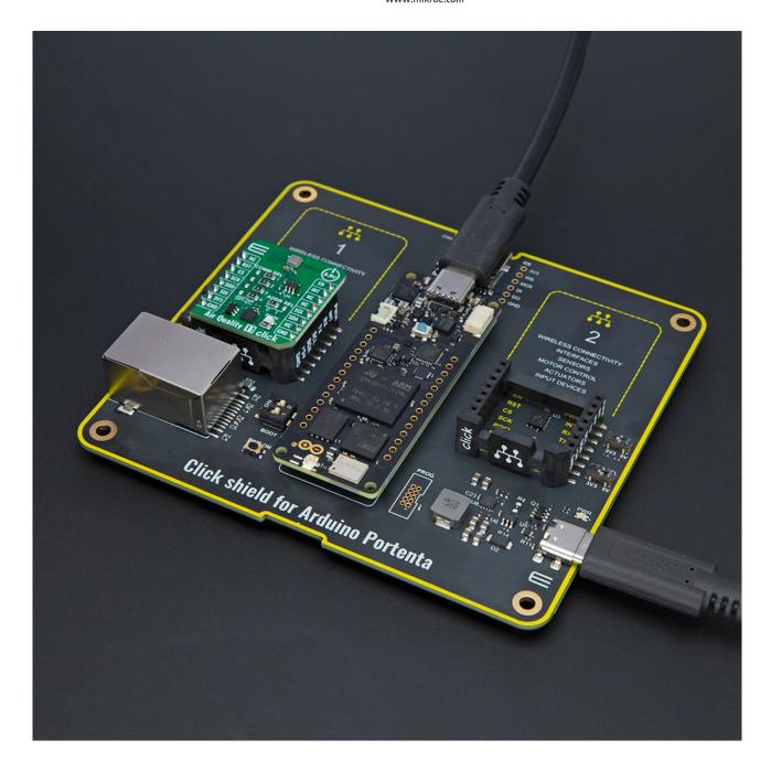
When the USB is connected to the Click Shield, and the other USB is connected to the Portenta board, the PWR diode will glow Cyan, and at this setup, the mikroBUS $^{\text{m}}$  sockets are powered from the Type C connector from Click Shield.
