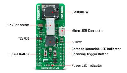
The EM3080-W scanner module uses a flat cable to connect to the Click board<sup>™</sup>, via the FPC Connector which is located on the top side of the PCB. This flat cable carries all the signals used in communication between the EM3080-W module and the host MCU, such as the RX, TX, buzzer, USB, LED, reset, and scanning trigger lines.
