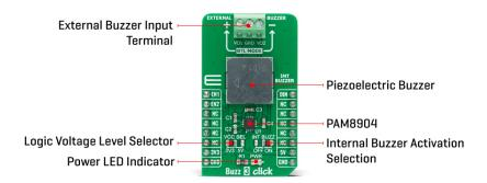
The sounder driver helps to keep current consumption low and battery life long by employing built-in automatic shutdown and wake-up functions. For example, active current consumption is just  $300\mu A$  in 1x mode, with an input voltage of 3V, input frequency of 4kHz, and driving a 15nF piezo. In shutdown mode, the quiescent current is less than  $1\mu A$ .
