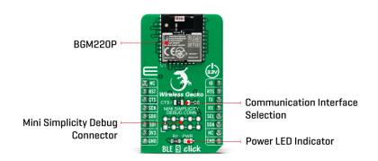
The EFR32BG22 SoC, inside the BGM220P module, includes an Arm Cortex-M33 processing core, up to 32Kb of RAM, up to 512kB of flash memory, and a 2.4GHz radio transceiver, offering up to 8dB output power. This Click board  $^{\text{TM}}$  offers enhanced performance, security, and reliability to support IoT products running on Bluetooth networks.
