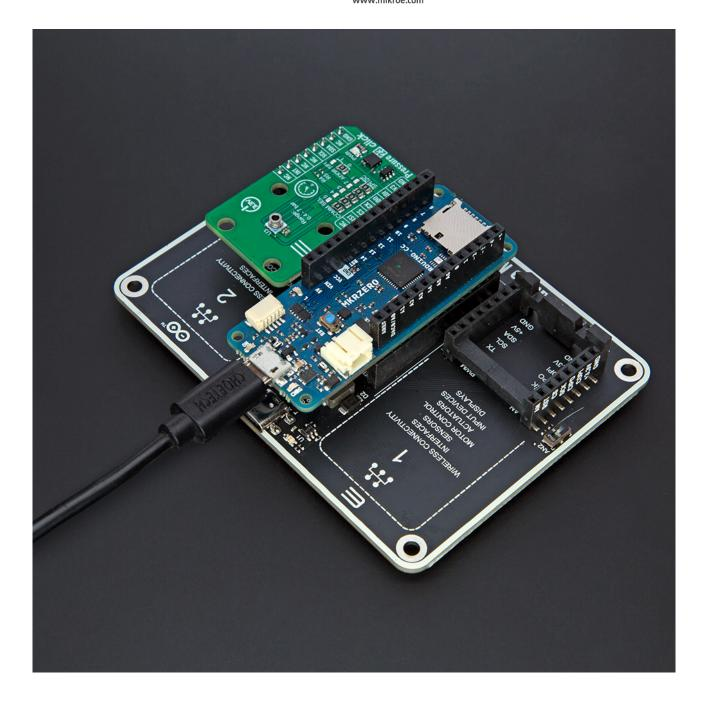
When the USB is connected to the Arduino MKR board, the PWR diode will glow Green, and at this setup, the Arduino MKR baseboard itself will be powered and will provide power to the Shield including two mikroBUS $^{\text{m}}$  sockets.
