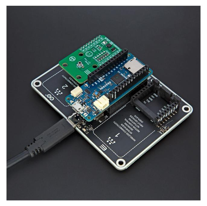
When the USB type C connector is connected to the Shield, the PWR diode will glow Blue, and at this setup, the connected Arduino MKR baseboard and two mikroBUS $^{\text{m}}$  sockets will be powered from it.
