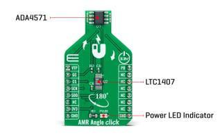
The ADA4571 contains two Wheatstone bridges, at a relative angle of 45° to one another. A rotating magnetic field in the x-y sensor plane delivers two sinusoidal output signals with the double frequency of the angle between sensor and magnetic field direction. Within a homogeneous field in the x-y plane, the output signals are independent of the physical placement in the z-direction (air gap).
