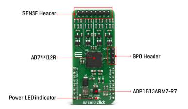
The ADC can measure either the voltage across the  $100~\Omega$  RSENSE or the voltage at the I/OP\_x screw terminal of each channel. In high impedance mode, the ADC, by default, measures the voltage across the screw terminals (I/OP\_x to I/ON\_x) in a 0 V to 10 V range. The ADC also provides diagnostic information on user-selectable inputs such as supplies, internal die temperature, reference, and regulators.
