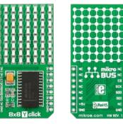
8x8 Y Click<sup>™</sup> is an accessory board in mikroBUS<sup>TM</sup> form factor. It's a compact and easy solution for adding 8x8 YELLOW LED matrix to your design. It features MAX7219 8-digit LED display driver module as well as 64 YELLOW LED diodes. 8x8 Y Click<sup>™</sup> communicates with target board microcontroller via four mikroBUS<sup>TM</sup> SPI lines (DIN, DOUT, CLK and CS). The board is designed to use 5V power supply only, but it can be used with 3.3V MCUs as well.
