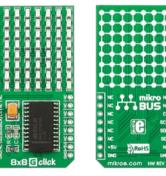
8x8 G Click<sup>™</sup> is an accessory board in **mikroBUS**<sup>Th</sup> form factor. It's a compact and easy solution for adding 8x8 GREEN LED matrix to your design. It features MAX7219 8-digit LED display driver module as well as 64 GREEN LED diodes. 8x8 G Click<sup>™</sup> communicates with target board microcontroller via four mikroBUS<sup>™</sup> SPI lines (DIN, DOUT, CLK and CS). The board is designed to use 5V power supply only, but it can be used with 3.3V MCUs as well.
