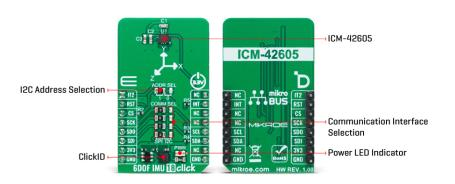
The gyroscope supports eight programmable full-scale range settings from  $\pm 15.625$  dps to  $\pm 2000$  dps, and the accelerometer supports four programmable full-scale range settings from  $\pm 2q$  to  $\pm 16q$ . Other industry-leading features include on-chip 16-bit ADCs, programmable digital filters, an embedded temperature sensor, and programmable interrupts. The ICM-42605 also provides high robustness by supporting 20,000g shock reliability.
