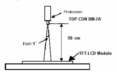
Note2: Measured at the center area of the panel and at the viewing angle of the  $\theta$  x=  $\theta$  y =0°
