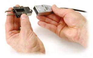
The micro design employs the use of tip cartridges with a twin parallel design, so the tips are always in alignment. With the WMRT, you are able to desolder very small SMD components down to 0201
