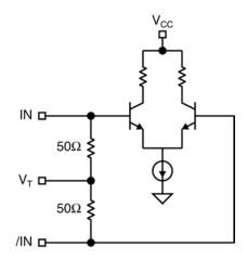
Figure 6. Simplified Differential Input Stage
