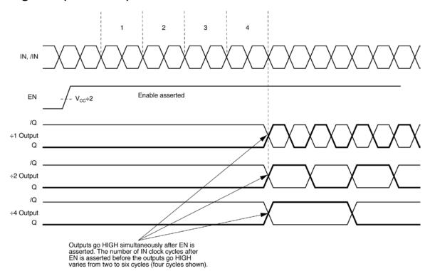
Figure 4. Enable Timing
