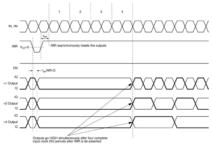
Figure 3. Reset with Output Enabled
