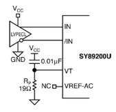
Figure 9. LVPECL Interface (DC-Coupled)
