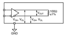
Figure 12. LVDS Differential Measurement
