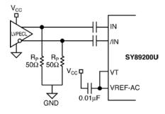
Figure 10. LVPECL Interface (AC-Coupled)
