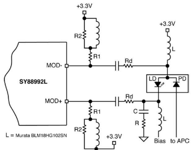
Figure 3. Driving a Common Anode VCSEL Differentially
