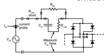
Do not connect earth-grounded instruments when operating off the AC line! Use either battery-powered equipment, high voltage differential probes, or an isolation transformer on the AC line. Note that many Variacs (variable transformers) do not provide isolation.
