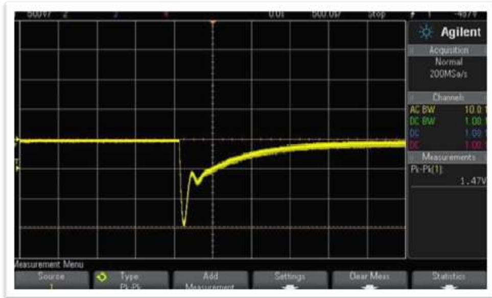
Figure 11: 12V/25W Flyback Output Voltage at Load Switching from 20% to 90%
