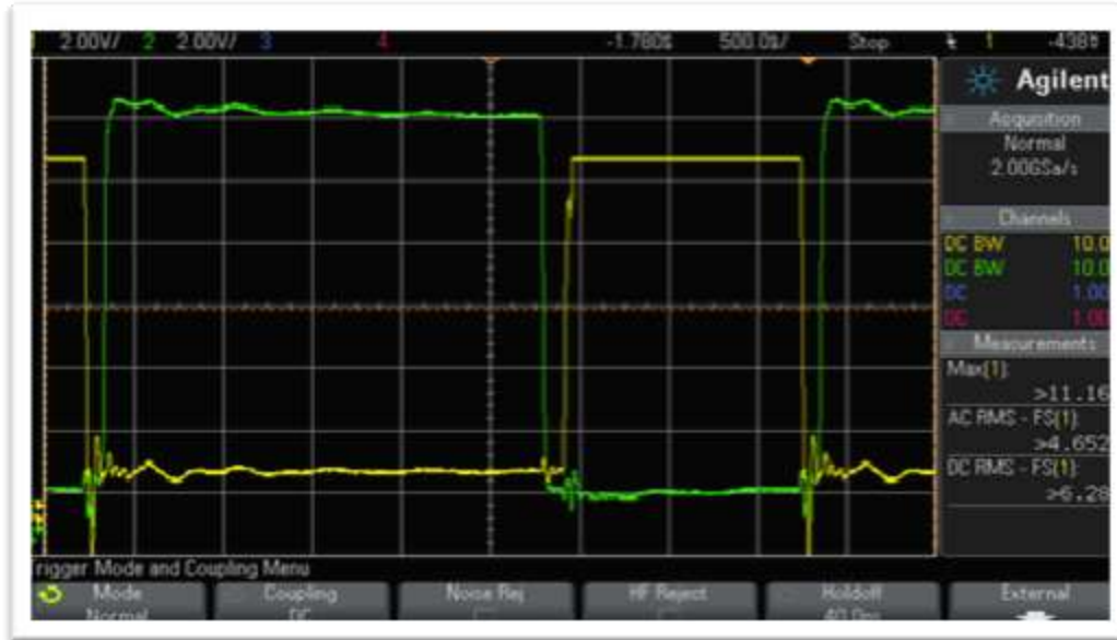
Figure 13: 12V/25W Flyback Primary and secondary Fets Gate
