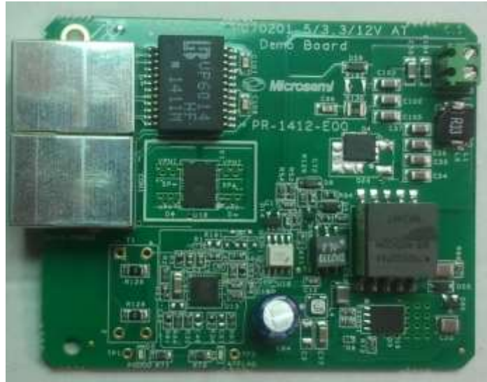
Figure 2: PD70201EVB25FX Evaluation Board – General View
