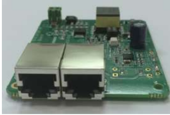
Figure 3: Front RJ45 and Wall Adapter Connectors
