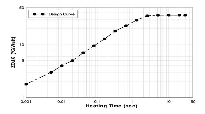
FIGURE 2. Thermal impedance graph  $R_{\theta JL}$  36°C/W.
