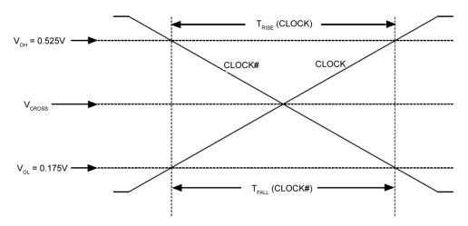
Figure 2. Single-Ended Measurement Points for  $T_{\text{RISE}}$  and  $T_{\text{FALL}}$
