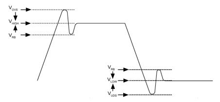
Figure 3. Single-Ended Measurement Points for  $V_{\text{OVS}},\,V_{\text{UDS}},\,\text{and}\,\,V_{\text{RB}}$
