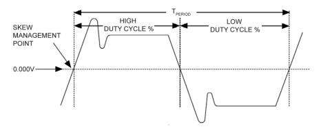
Figure 4. Differential (Clock/Clock#) Measurement Points for T<sub>PERIOD</sub>, Duty Cycle, and Jitter
