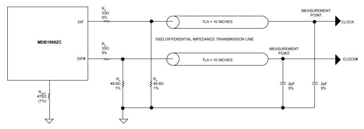
Figure 5. 0.7V Configuration Test Load Board Termination with  $100\Omega$  Differential Impedance Transmission Line
