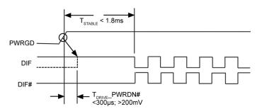
Figure 7. PWRGD Assertion (Power-Down De-Assertion)
