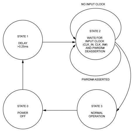
Figure 9. Buffer Power-Up State Diagram
