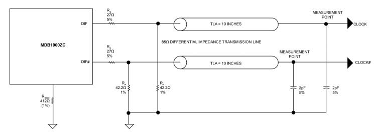
Figure 6. 0.7V Configuration Test Load Board Termination with  $85\Omega$  Differential Impedance Transmission Line
