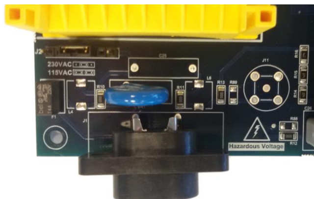
Figure 7-10. ATPL250ABN mains and voltage jumper selector.
