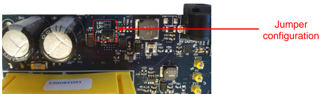
Figure 5-3. V DD selection in ATPL250ABN board.
