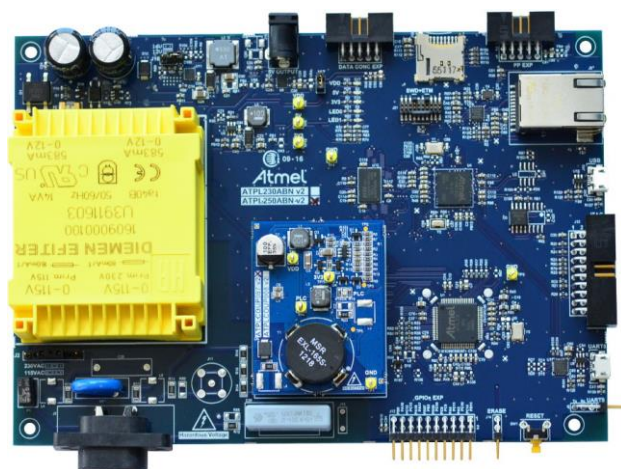
Figure 2-2. ATPL250ABN PAN Coordinator board and with ATPLCOUP007.
