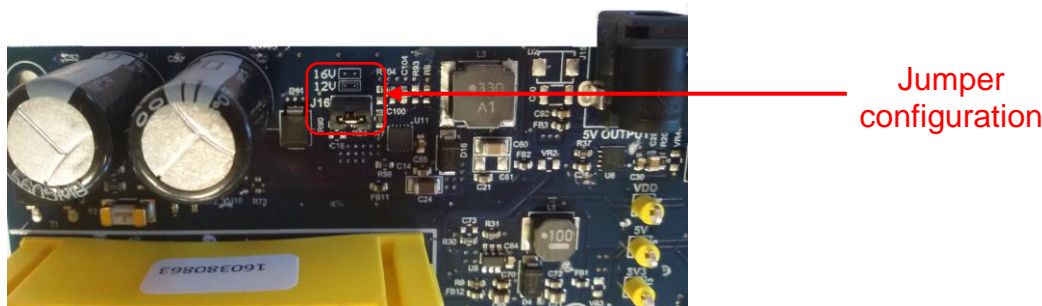
Figure 6-3. V DD selection in ATPL250ABN board.
