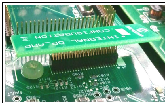
FIGURE 2: INTERNAL OP AMP CONFIGURATION BOARD
