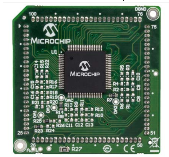
FIGURE 2: EXTERNAL OP AMP CONFIGURATION BOARD
