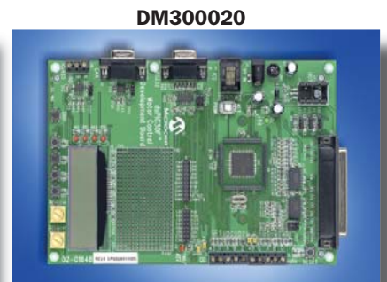
Includes a dsPIC30F6010 plug-in module (MA300013)
