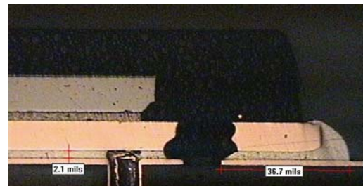
81% Paste Coverage, Encroached Via, 2.1 mil Standoff
