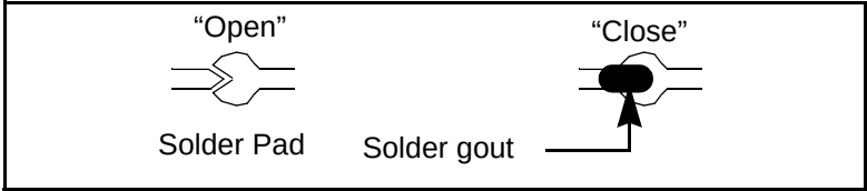
Figure 2-11. Solder Strap definition
