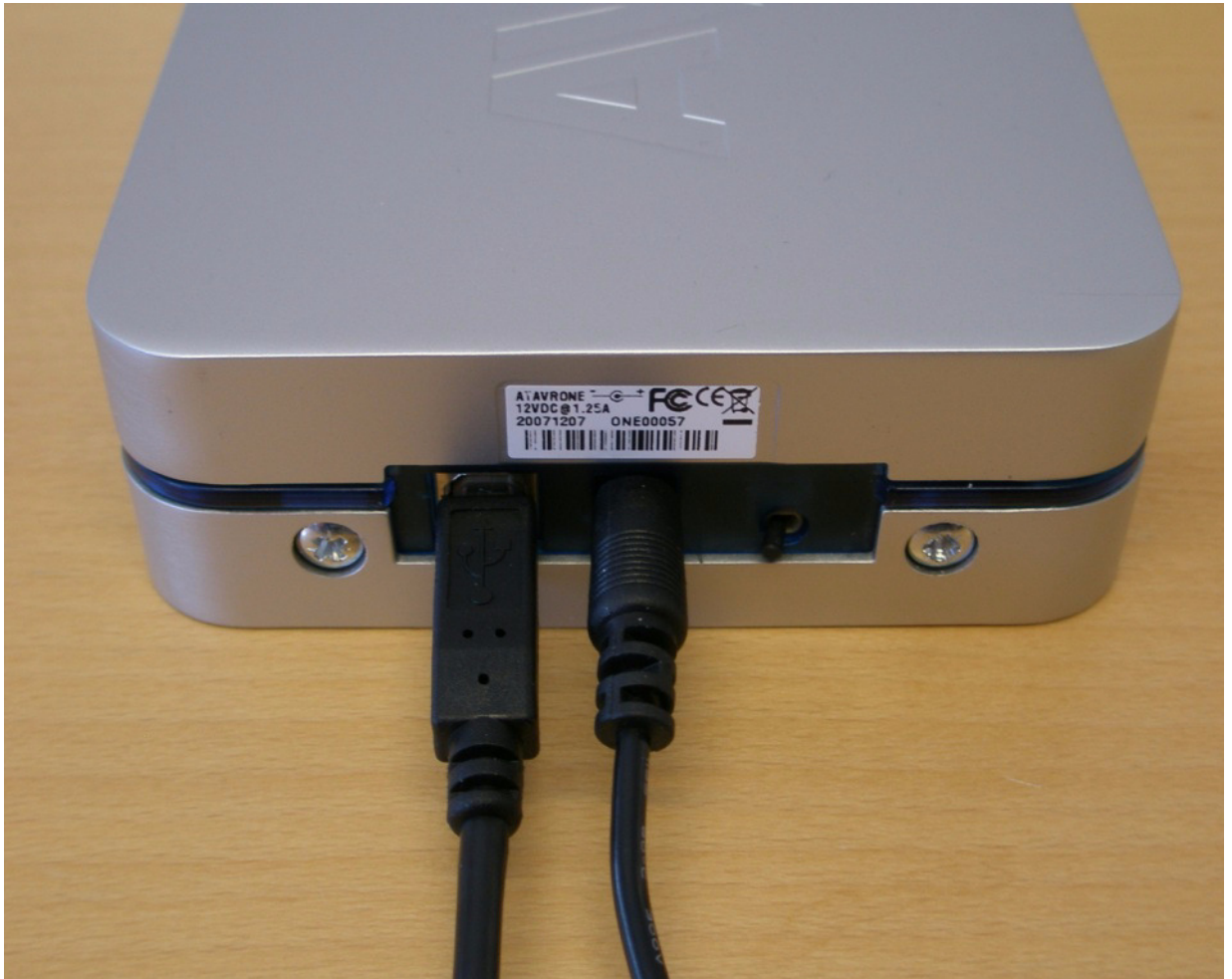
Figure 3-19. AVR ONE! connected to power and USB
