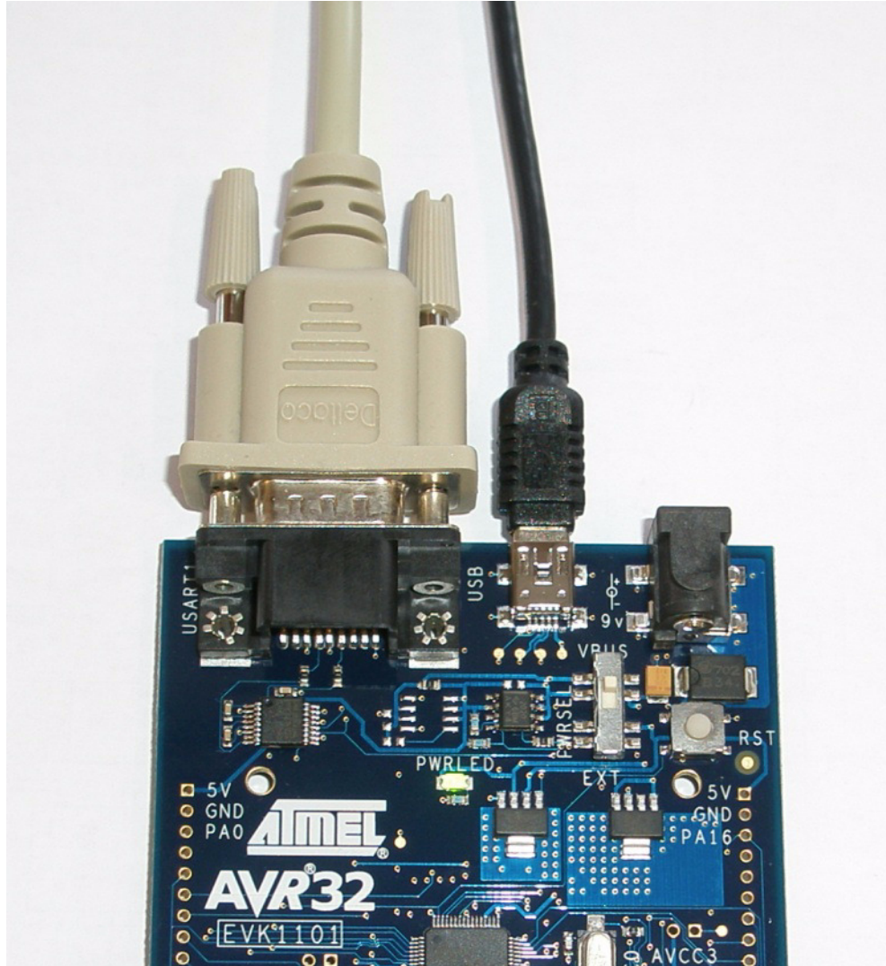
Figure 4-2. Powering the EVK1101 using the USB cable
