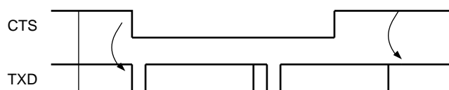
Figure 33-19. Transmitter Behavior when Operating with Hardware Handshaking
