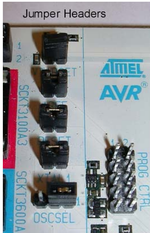
Figure 1-2. Detail of Jumper Placement on the STK500
