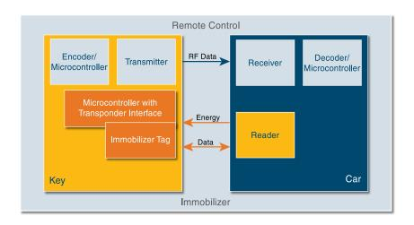
Bi-directional RF link for RKE functions as well as for the extremely secure duplex RF link in a Passive Entry Go (PEG) system. The LF link is used for the wake-up channel in a PEG system as well as for the immobilizer function to start the RF communication.
