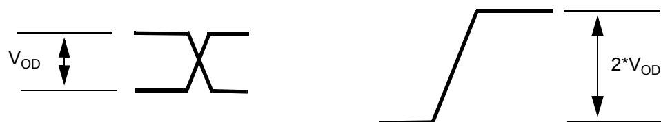
Figure 19 - Differential Output Voltage Parameter
