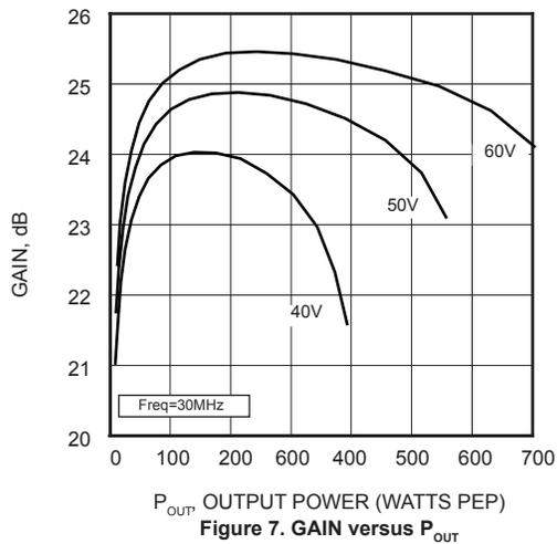
Figure 7. GAIN versus P<sub>OUT</sub>
