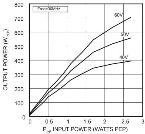
Figure 6. P<sub>OUT</sub> versus P<sub>IN</sub>
