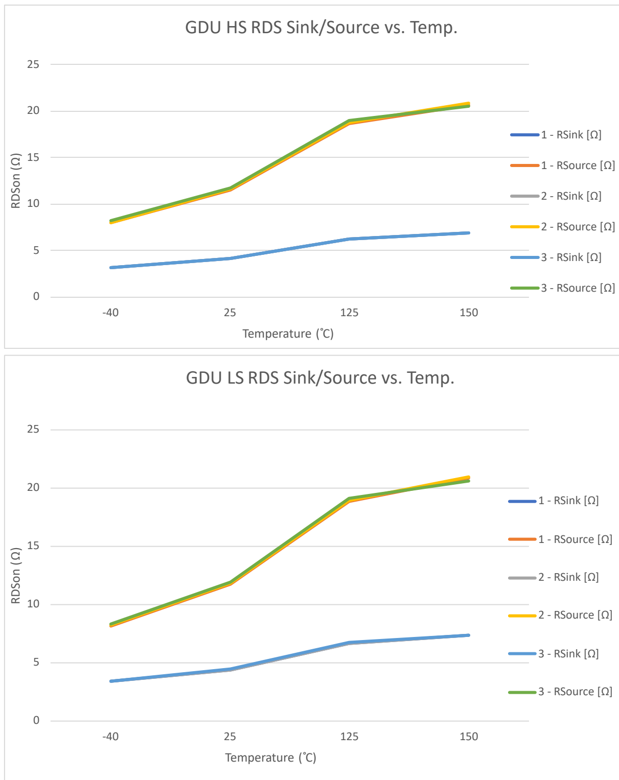
Figure 7-5. Gate Driver Unit Sink/Source ON Resistance vs Temperature
