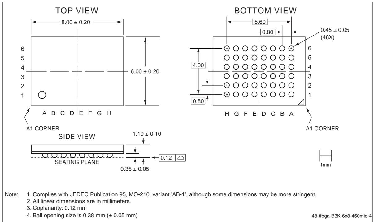
**Figure 23:** 48-Ball Very-Very-Thin-Profile, Fine-Pitch Ball Grid Array (WFBGA) 4mm x 6mm
