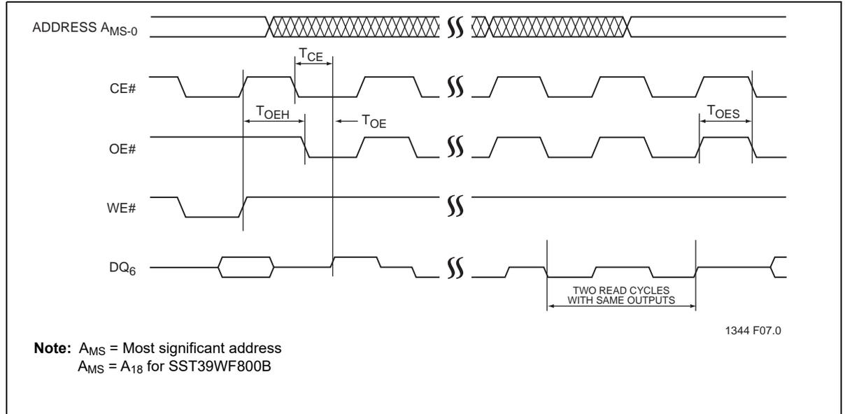
**Figure 10: WE# Controlled Chip-Erase Timing Diagram**
