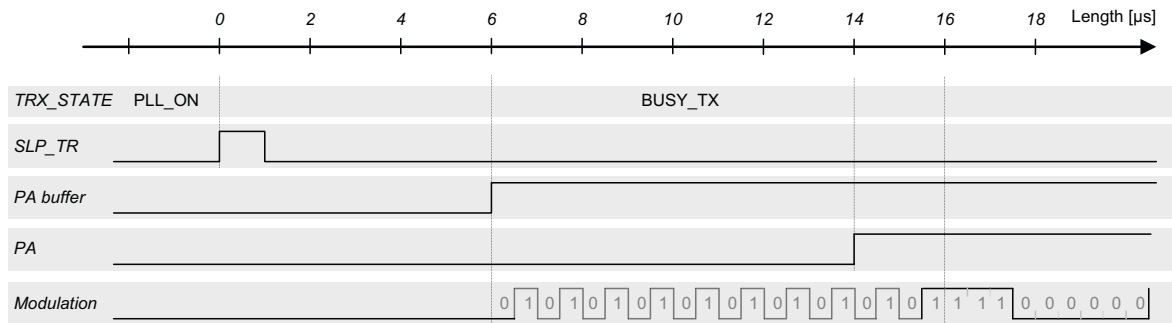
Figure 38-3. TX Power Ramping for Maximum TX Power
