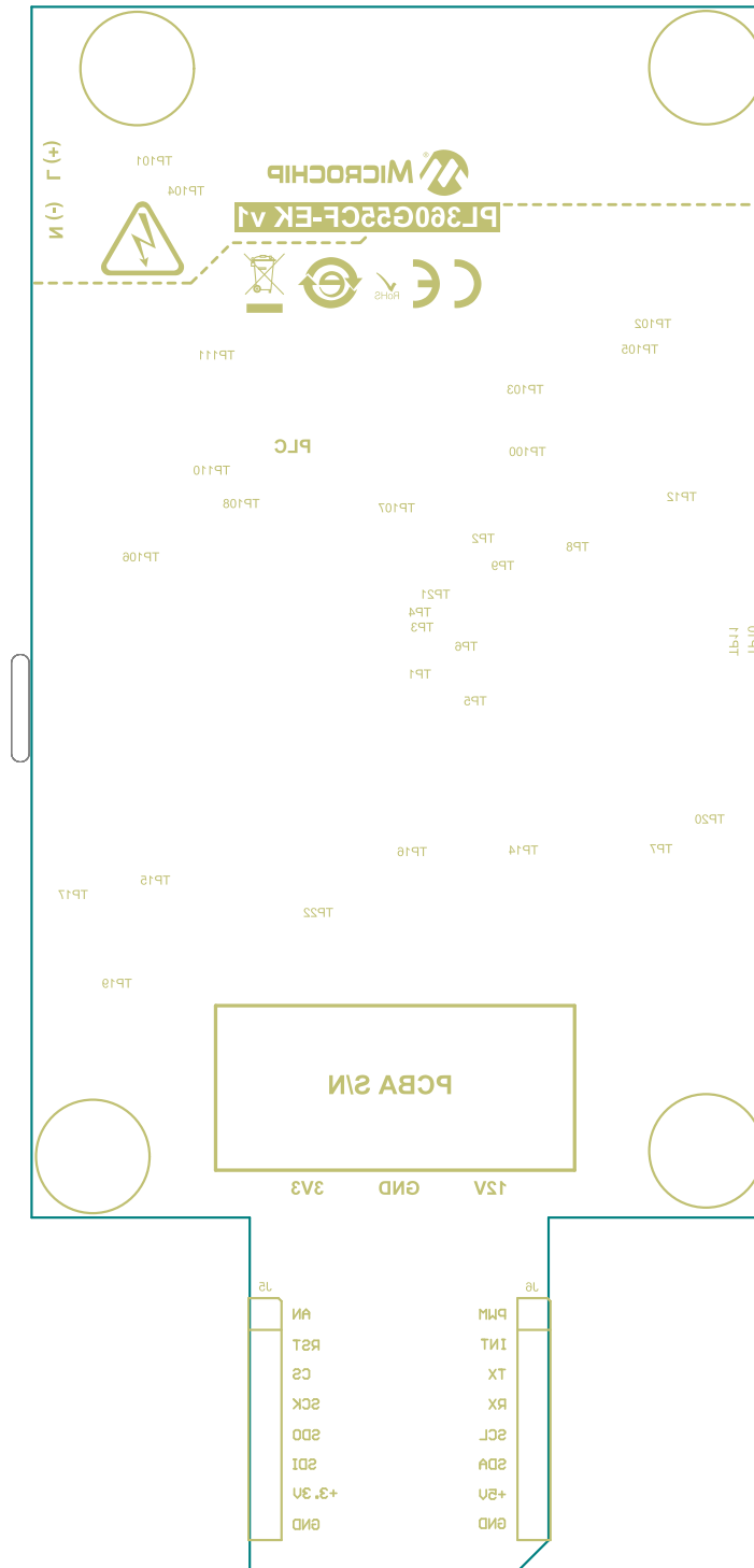
Figure 3-33. PL360G55CF-EKv1 Layout: Bottom Silkscreen
