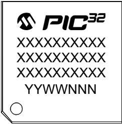
64-Lead TQFP (10x10x1 mm)
