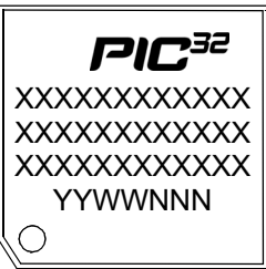
48-Lead VQFN (6x6x0.9 mm)
