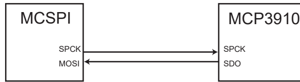
Figure 47-14. MCP3910 Basic Connection to MCSPI
