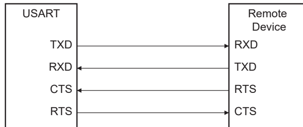
Figure 34-26. Connection with a Remote Device for Hardware Handshaking
