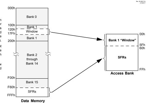
Remapping of the Access Bank applies only to operations using the Indexed Literal Offset mode. Operations that use the BSR (Access RAM bit is '1') will continue to use Direct Addressing as before.
