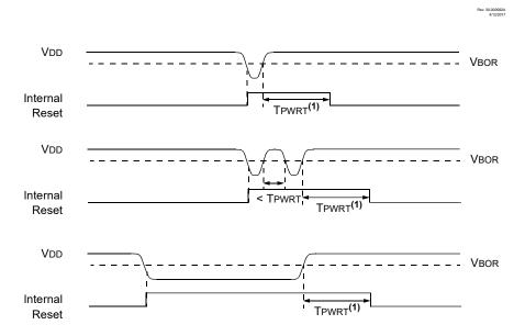
**Note:**  $T_{PWRT}$  delay only if the <u>PWRTE</u> bit is programmed to '0'.
