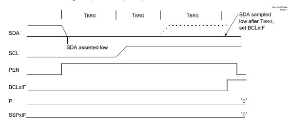
Figure 27-39. Bus Collision During a Stop Condition (Case 1)
