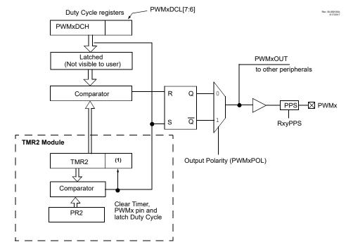
Note 1: 8-bit timer is concatenated with the two Least Significant bits of 1/Fosc adjusted by the Timer2 prescaler to create a 10-bit time base.
