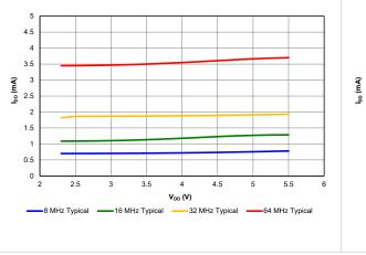
Figure 39-41. IDD, ECH Oscillator, Maximum
