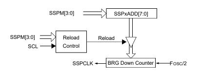
**Important:** Values of  $0 \times 00$ ,  $0 \times 01$  and  $0 \times 02$  are not valid for SSPxADD when used as a Baud Rate Generator for I<sup>2</sup>C. This is an implementation limitation.
