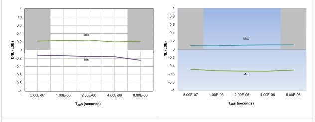
**Figure 39-9.** ADC 10-bit, DNL, V<sub>DD</sub> = 3.0V, T<sub>AD</sub> = 1 μs, Min **Figure 39-10.** ADC 10-BIT, INL, V<sub>DD</sub> = 3.0V, T<sub>AD</sub> = 1 μs, and Max values at 125°C + 3σ Min and Max values at 125°C +  $3\sigma$
