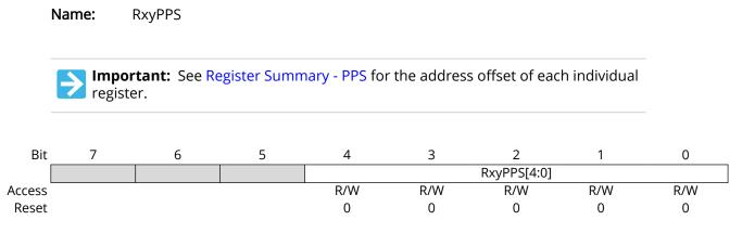
**Bits 4:0 – RxyPPS[4:0]** Pin Rxy Output Source Selection bits See the *"Peripheral PPS Output Selection Codes"* table for details about source selection.
