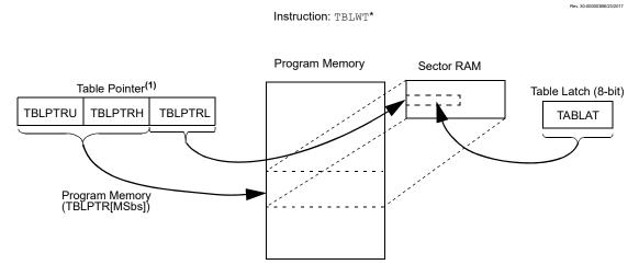
**Note** 1: During table writes the Table Pointer points to two areas. The LSbs of TBLPRTL point to an address within the sector RAM space. The MSbs of the Table Pointer determine where the sector will eventually be written.
