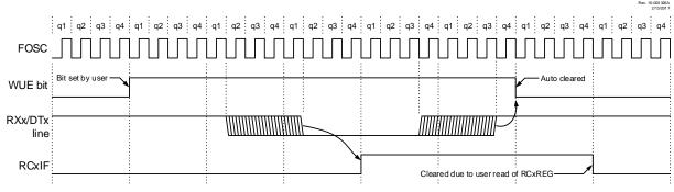
Figure 28-7. Auto-Wake-Up (WUE) Bit Timing During Normal Operation
