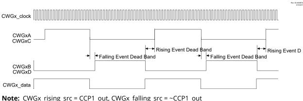
Figure 25-1. CWG Half-Bridge Mode Operation
