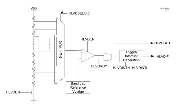
Since the HLVD can be software enabled through the HLVDEN bit, setting and clearing the enable bit does not produce a false HLVD event glitch. Each time the HLVD module is enabled, the RDY bit can be used to detect when the module is stable and ready to use.
