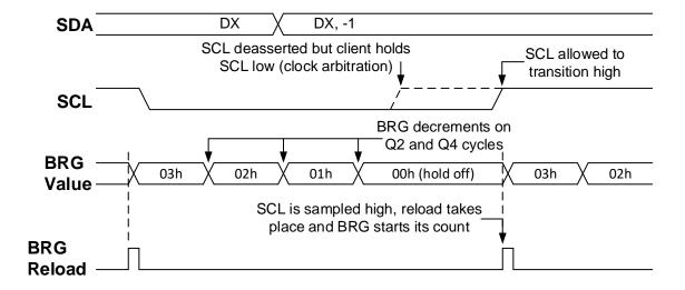
Figure 27-24. Baud Rate Generator Timing with Clock Arbitration
