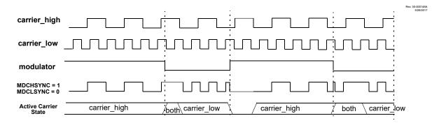
**Figure 26-5.** Carrier Low Synchronization (MDCHSYNC = 0, MDCLSYNC = 1)
