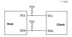
The I<sup>2</sup>C bus can operate with one or more host devices and one or more client devices.
