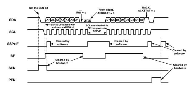
Figure 27-29. I<sup>2</sup>C Host Mode Waveform (Transmission, 7-Bit Address)
