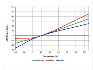
Figure 39-71. Temperature Indicator Slope Normalized to 20°C, High Range,  $V_{DD}$  = 3.5V
