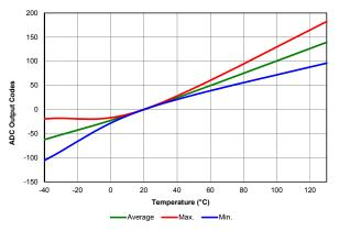
Figure 39-72. Temperature Indicator Slope Normalized to 20°C, High Range,  $V_{DD}$  = 3.0V
