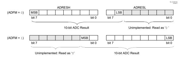
Figure 32-3. 10-Bit ADC Conversion Result Format
