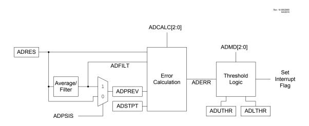
The operation of the ADC computational features is controlled by the ADMD bits.
