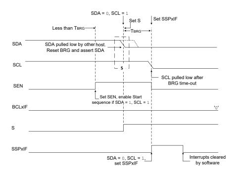
**Important:** The reason that a bus collision is not a factor during a Start condition is that no two bus hosts can assert a Start condition at the exact same time. Therefore, one host will always assert SDA before the other. This condition does not cause a bus collision because the two hosts must be allowed to arbitrate the first address following the Start condition. If the address is the same, arbitration must be allowed to continue into the data portion, Repeated Start or Stop conditions.
