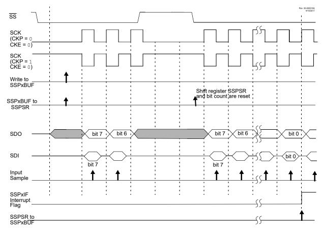
Figure 27-6. Client Select Synchronous Waveform
