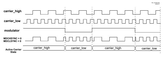
Figure 26-4. Carrier High Synchronization (MDCHSYNC = 1, MDCLSYNC = 0)
