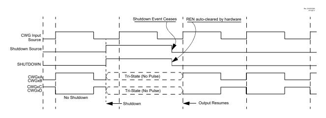
Figure 25-16. Shutdown Functionality, Auto-Restart Enabled (REN = 1, LSAC = 01, LSBD = 01)
