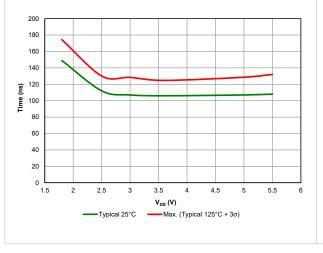
Figure 39-28. Comparator Response Time Rising edge
