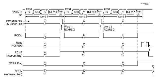
Figure 28-5. Asynchronous Reception
