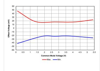
**Figure 39-26.** Comparator Offset, Normal Power Mode (CxSP = 1), Vdd = 5.5V, Measured Values From -40°C to 125°C
