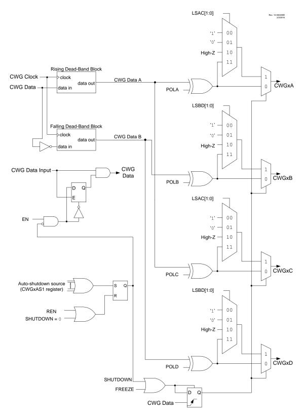
Figure 25-2. Simplified CWG Block Diagram (Half-Bridge Mode, MODE[2:0] = 100)
