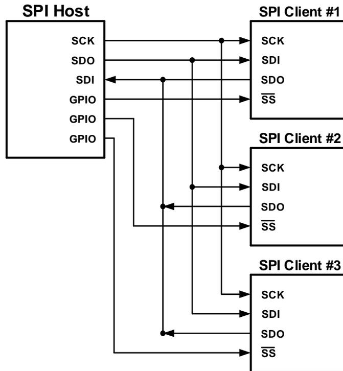
Transmissions involve two shift registers, eight bits in size: One in the host and one in the client. Data are shifted out one bit at a time, with the Most Significant bit (MSb) shifted out first. At the same time, a new Least Significant bit (LSb) is shifted into the same register.
