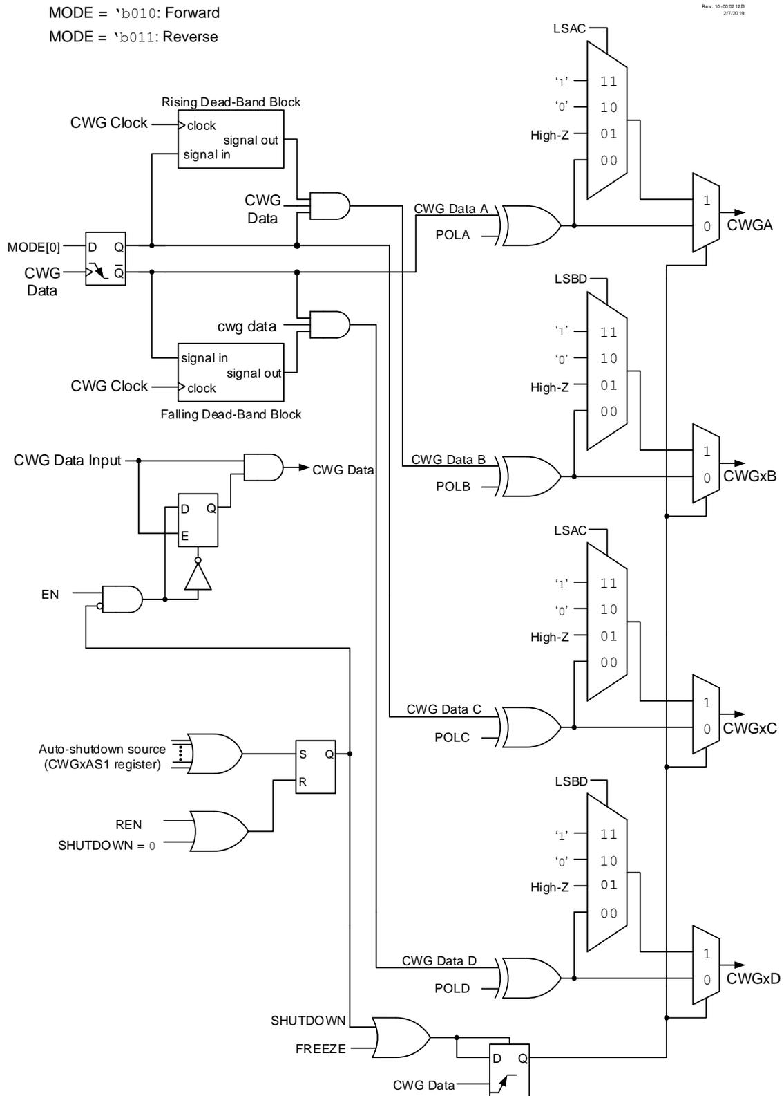
In Forward Full Bridge mode ( $MODE = \text{'b}010$ ), CWGxA is driven to its Active state, CWGxB and CWGxC are driven to their Inactive state, and CWGxD is modulated by the input signal, as shown in Figure 23-7.
