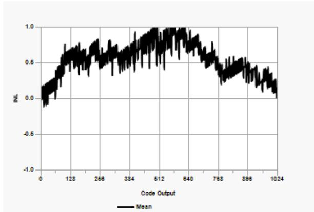
**Figure 42-5.** ADC, INL,  $V_{DD} = 3.0V$ ,  $T_{AD} = 4 \mu s$
