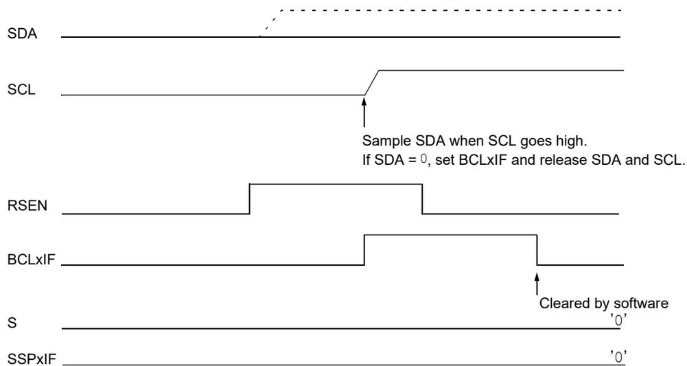
If SCL goes from high-to-low before the BRG times out and SDA has not already been asserted, a bus collision occurs. In this case, another host is attempting to transmit a data '1' during the Repeated Start condition (see [Figure 29-38](#)).
