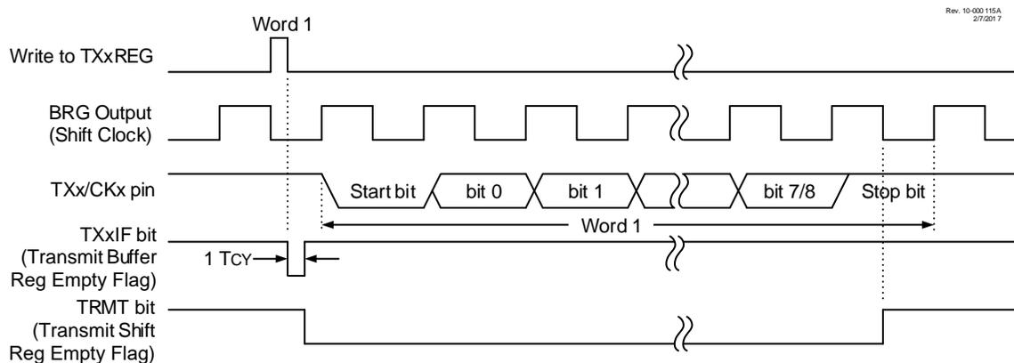
**Figure 30-4.** Asynchronous Transmission (Back-to-Back)
