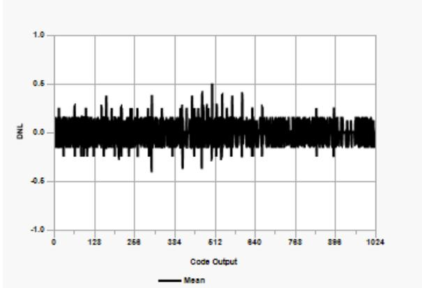
**Figure 42-2.** ADC, DNL,  $V_{DD} = 3.0V$ ,  $T_{AD} = 4 \mu s$
