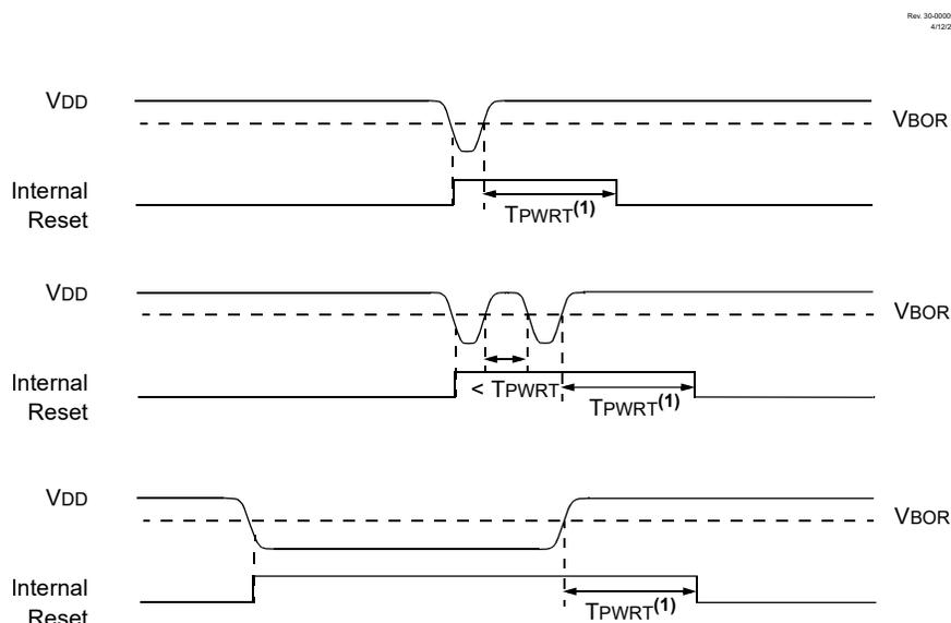
**Note:**  $T_{PWRT}$  delay when the PWRTS bits are enabled ( $\overline{PWRTS} \neq 00$ ).
