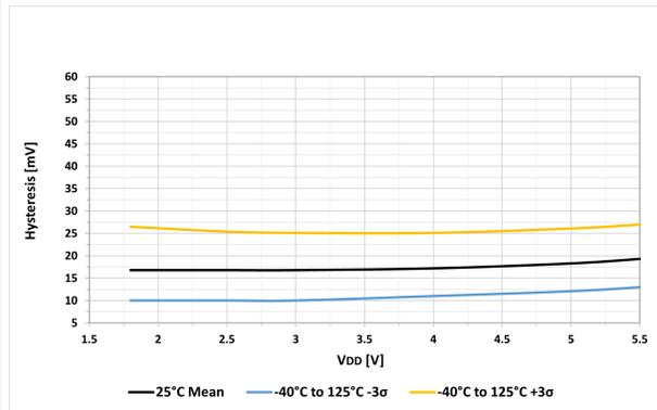
**Figure 42-13.** Comparator Hysteresis, Hysteresis Disabled ( $CxHYS = 0, V_{ICM} = V_{DD}/2$ )
