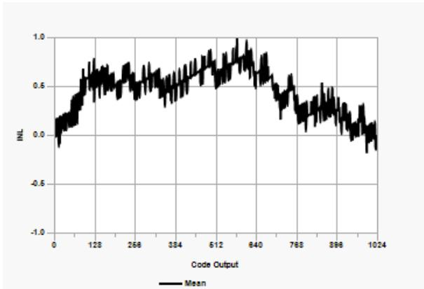
**Figure 42-6.** ADC, INL,  $V_{DD} = 3.0V$ ,  $T_{AD} = 8 \mu s$
