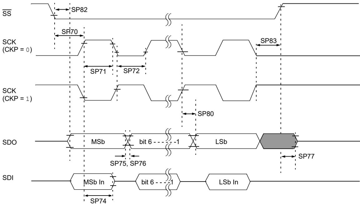
**Note:** Refer to the “Load Conditions” figure for load conditions.
