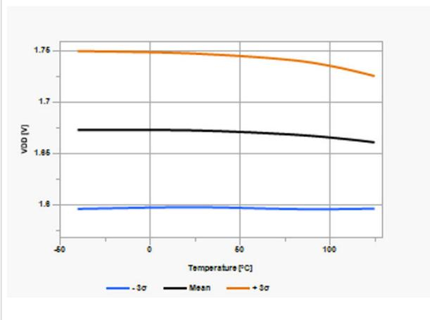
**Figure 42-51. POR Rearm Voltage**
