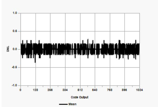
**Figure 42-3.** ADC, DNL,  $V_{DD} = 3.0V$ ,  $T_{AD} = 8 \mu s$
