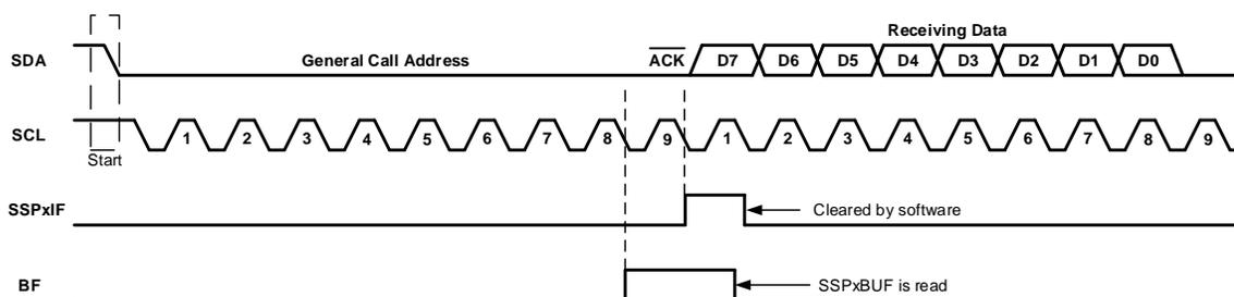
In 10-bit Address mode, the **UA** bit will not be set on the reception of the general call address. The client will prepare to receive the second byte as data, just as it would in 7-bit mode.
