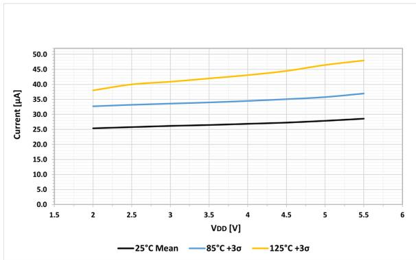
**Figure 42-42.**  $I_{PD}$ , Comparator (SP = 1, CPON = 00)
