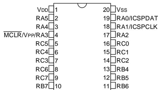
Figure 2-4. 20-Pin QFN, VQFN
