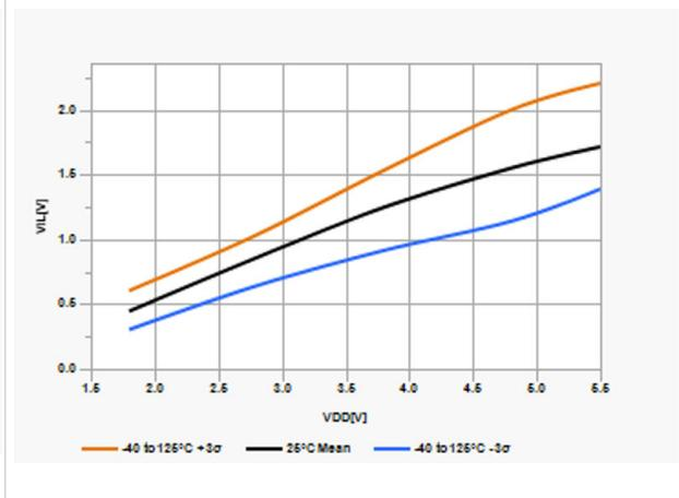
**Figure 42-36. TTL Input Level**
