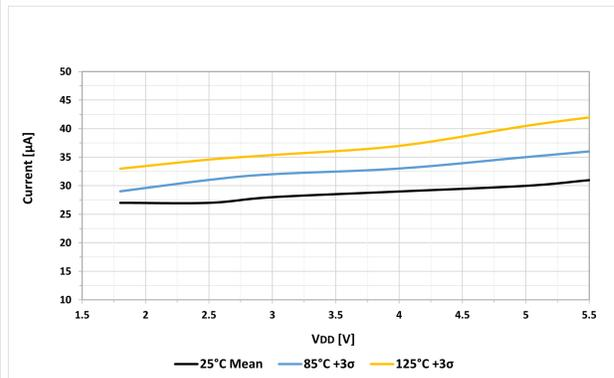
**Figure 42-43.**  $I_{PD}$ , Comparator (SP = 0, CPON = 00)
