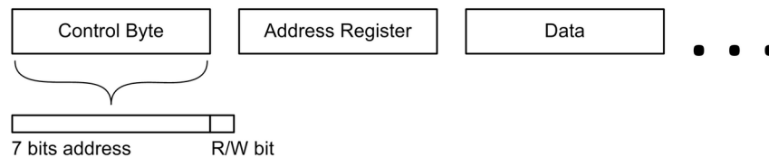
Figure 1-3. High-Level Packet Structure
