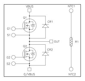
$V_{DSS} = 700V$   $R_{DSon} = 2.5 m\Omega \text{ typ } @ \text{Tj} = 25^{\circ}\text{C}$   $I_D = 689 * A @ \text{Tc} = 25^{\circ}\text{C}$
