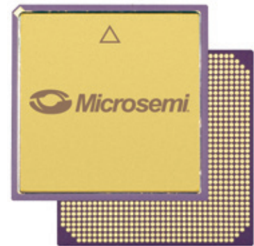
CG1272/LG1272 RTAX4000S, RTAX4000SL, and RTAX2000D only b.s. 1.457x1.457" (37.00x37.00 mm) h. CCGA - 218 mils (5.535 mm) h. CLGA - 129 mils (3.28 mm) p. 39 mils (1.00 mm)
