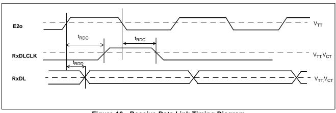
Figure 16 - Receive Data Link Timing Diagram
