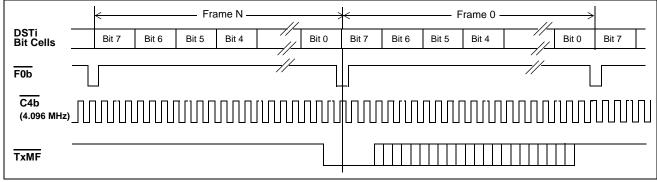
Figure 28 - Transmit Multiframe Functional Timing
