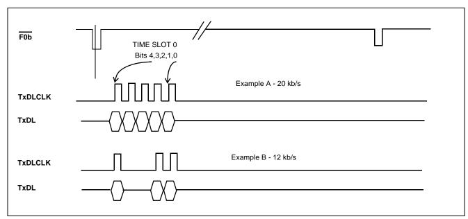
Figure 13 - Transmit Data Link Functional Timing
