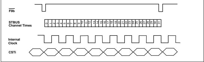
Figure 17 - Transmit 64 k Common Channel Functional Timing
