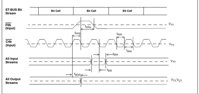
Figure 25 - GCI Timing Diagram (Input Clocks)
