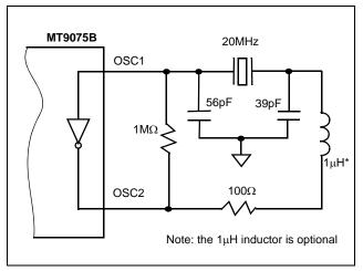
Figure 7 - Crystal Oscillator Circuit
