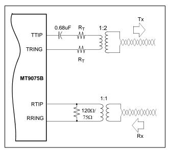
Figure 4 - Analog Line Interface
