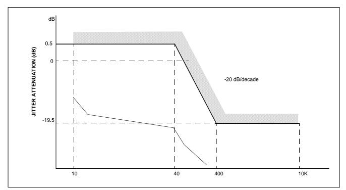
Figure 8 - Typical Jitter Attenuation Curve
