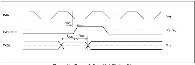
Figure 14 - Transmit Data Link Timing Diagram
