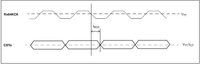
Figure 20 - Receive 64 k Common Channel Timing Diagram
