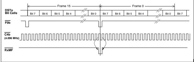
Figure 27 - Receive Multiframe Functional Timing
