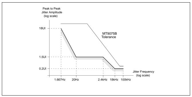
Figure 3 - Typical Jitter Tolerance
