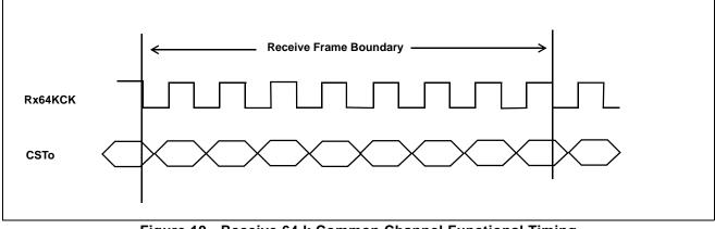
Figure 19 - Receive 64 k Common Channel Functional Timing
