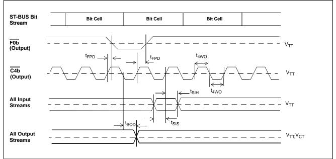
Figure 23 - ST-BUS Timing Diagram (Output Clocks)
