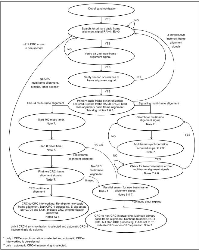
Figure 10 - Synchronization State Diagram
