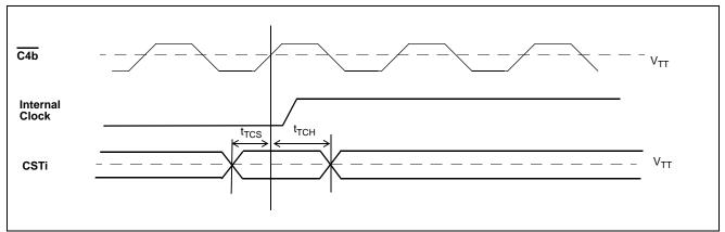
Figure 18 - Transmit 64 k Common Channel Timing Diagram
