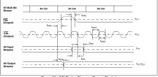
Figure 26 - GCI Timing Diagram (Output Clocks)
