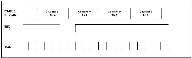
Figure 21 - ST-BUS Functional Timing Diagram
