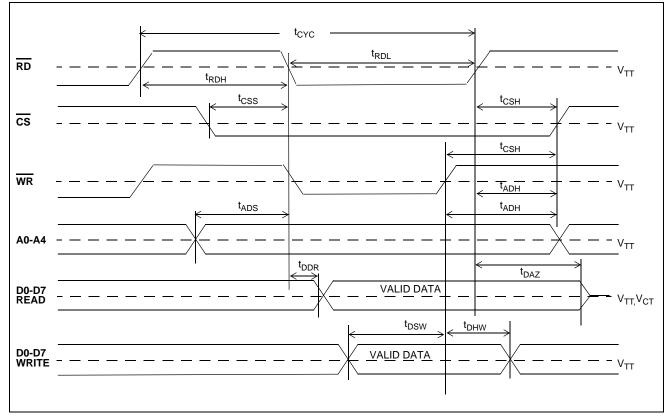
Figure 12 - Intel Microprocessor Timing
