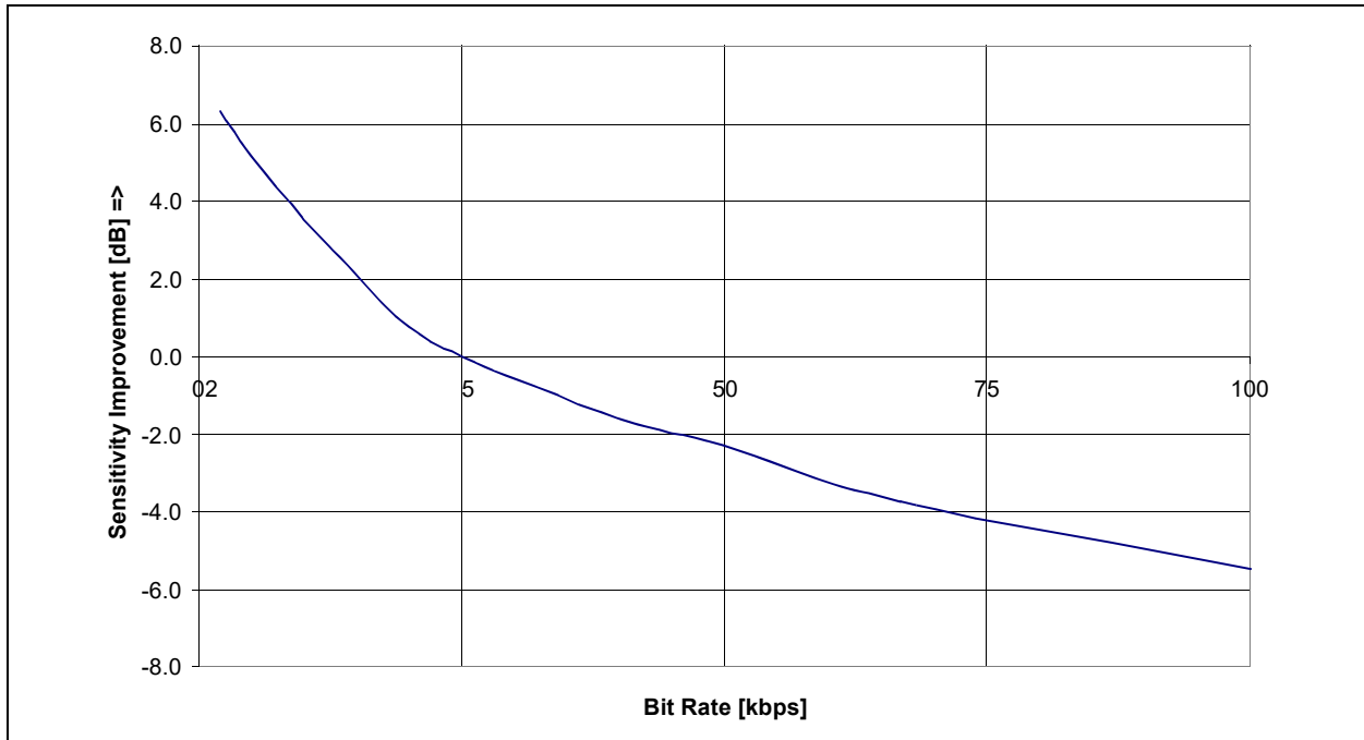
FIGURE 5-13: FSK SENSITIVITY VS. BR
