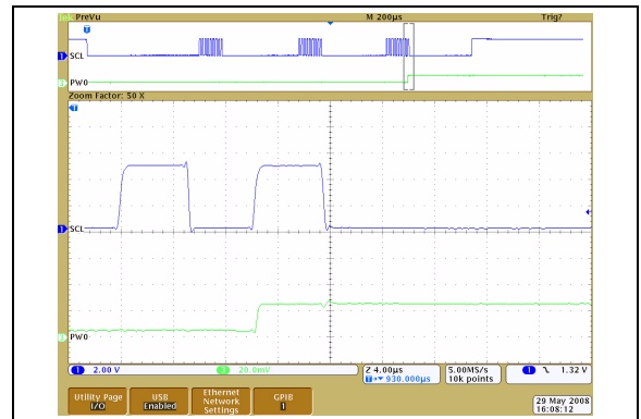
FIGURE 2-51: 50\text{ k}\Omega – Low-Voltage Increment Wiper Settling Time ( V_{DD} = 5.5\text{V} ) ( 1\text{ }\mu\text{s/Div} ).
