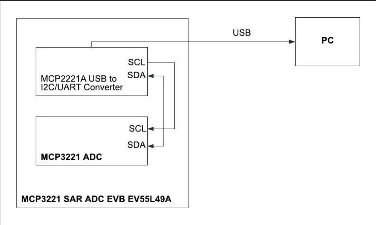
**FIGURE 2-5:** Diagram Connection between MCP3221 SAR ADC Evaluation Board and the PC by using MCP2221A.
