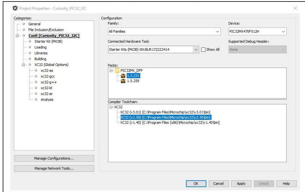
**FIGURE 4-2:** MPLAB IDE Settings.
