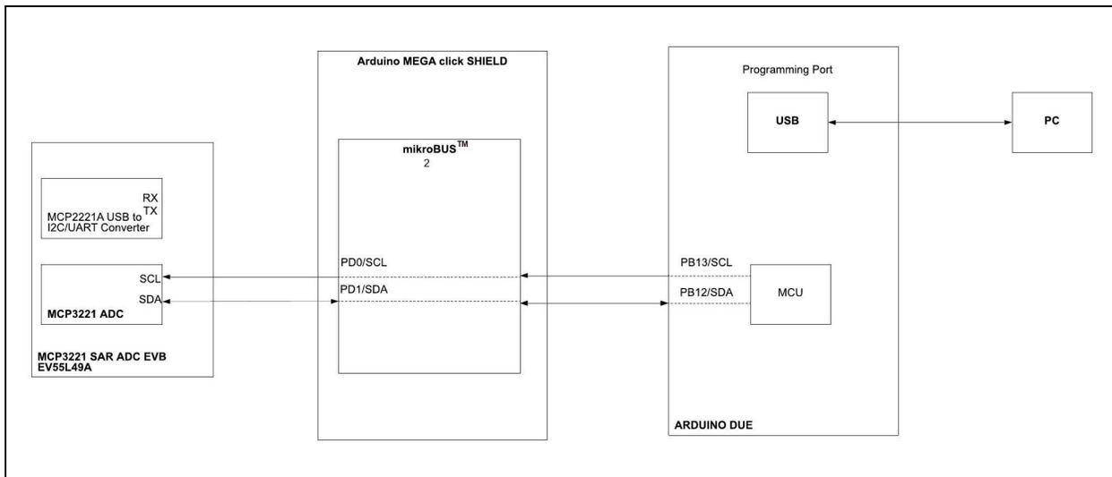
**FIGURE 2-3:** Diagram Connection between the MCU and the MCP3221 – Arduino Due Board.
