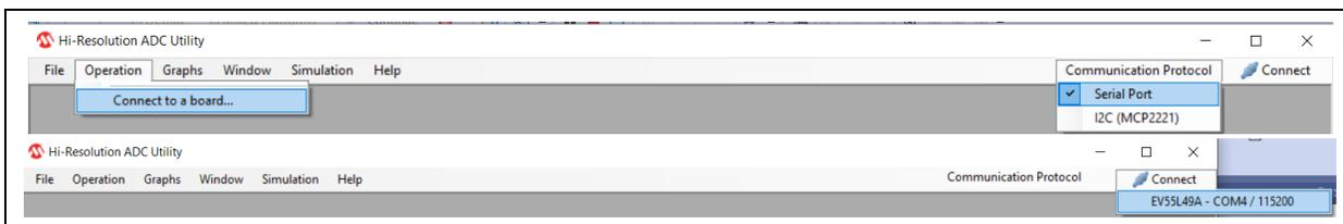
**FIGURE 4-7:** Connect Procedure for PIC32MX470F512H/Arduino Due Board.
