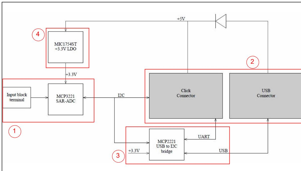
**FIGURE 2-2:** MCP3221 SAR ADC Evaluation Board – Diagram Block.
