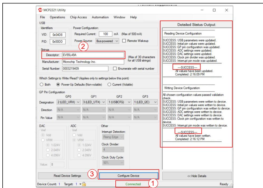
**FIGURE 4-5:** MCP2221A Utility Configuration Steps.
