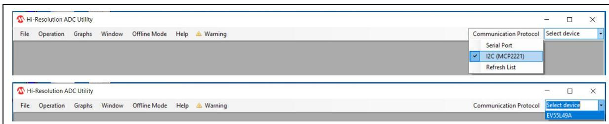
**FIGURE 4-8:** Connect Procedure for MCP3221 SAR ADC Evaluation Board using MCP2221A.
