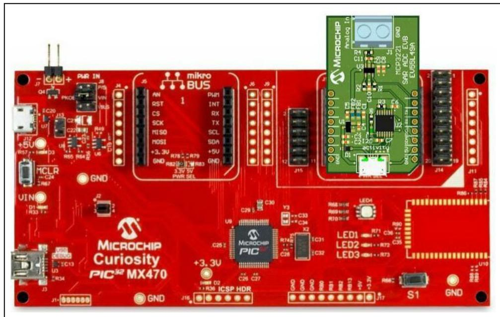
**FIGURE 4-1:** Hardware Connection of the MCP3221 SAR ADC Evaluation Board into the PIC32MX470 Curiosity Development Board.
