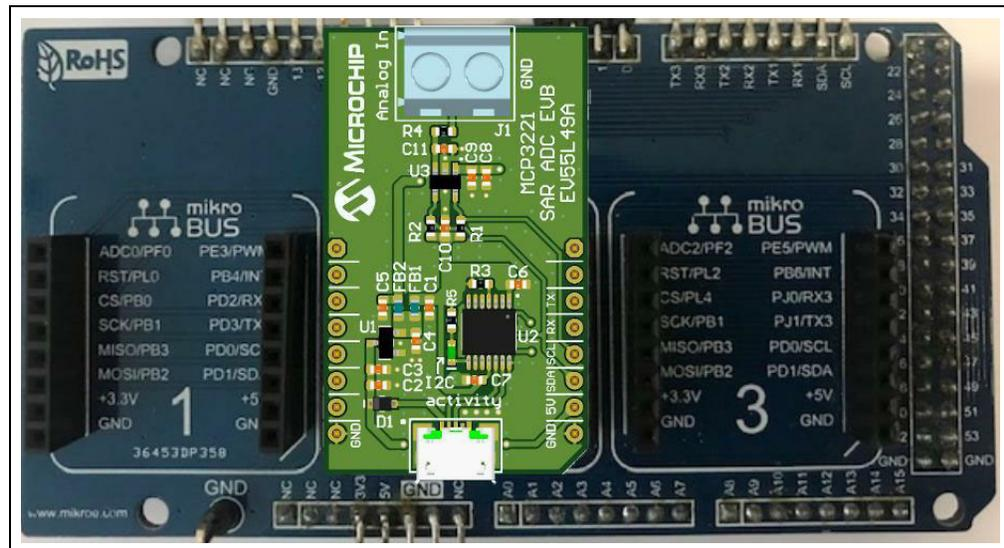
**FIGURE 4-3:** Hardware Connection of the MCP3221 SAR ADC Evaluation Board into the Arduino Due Board.
