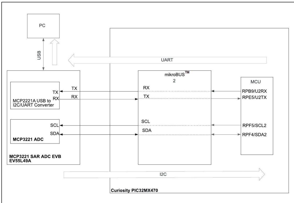
**FIGURE 2-4:** Diagram Connection between the MCU and MCP3221 – PIC32MX470 Curiosity Development Board.
