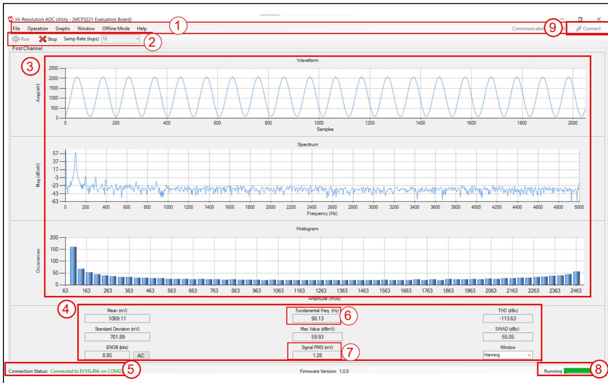
**FIGURE 4-9:** Hi-Resolution ADC Utility GUI – Main Window.
