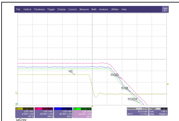
FIGURE 1-18: Typical LATCHC to HV_{OUT} Propagation Delay
