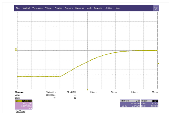
FIGURE 1-8: Typical HV_{OUT} from -135V to 0V, Load = 100 pF.
