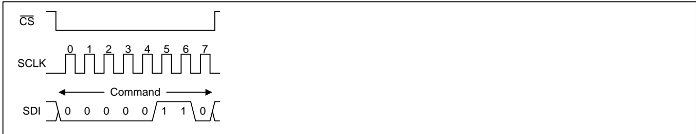
Figure 5-12. SPI Write Enable Transaction Functional Timing
