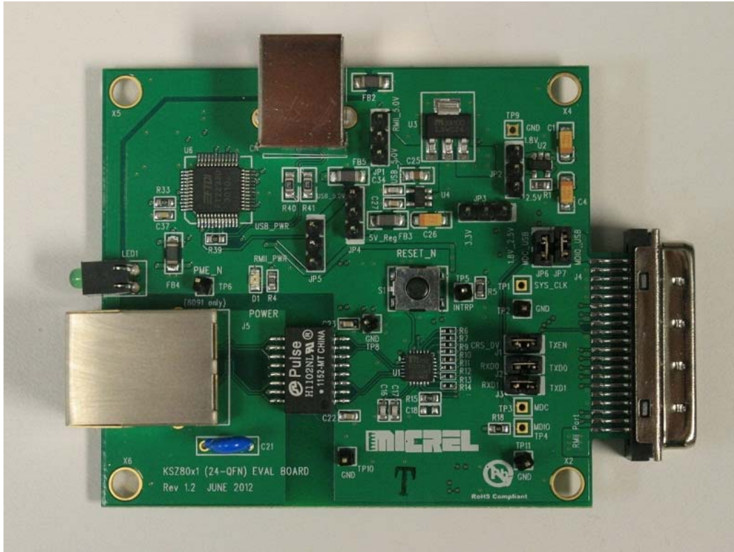
Figure 1. KSZ8081RNA / KSZ8081RND Evaluation Board
