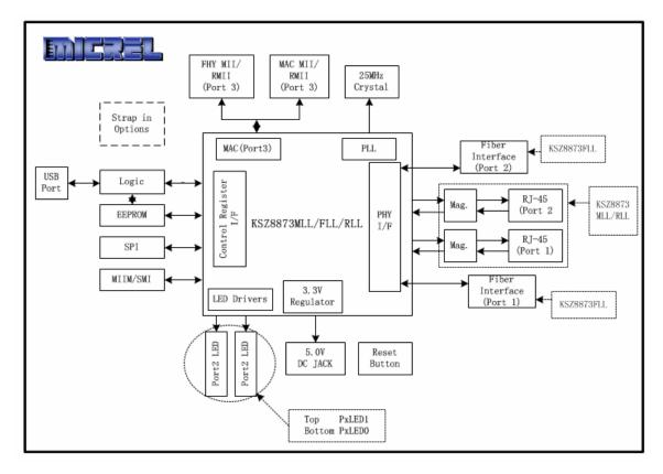
Figure 1: KSZ8873MLL/FLL/RLL Evaluation Board Block Diagram
